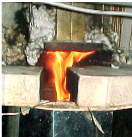
Fig. 6. Burning of resin at 500 °C, diameter 12.7 mm GFRP specimen.
