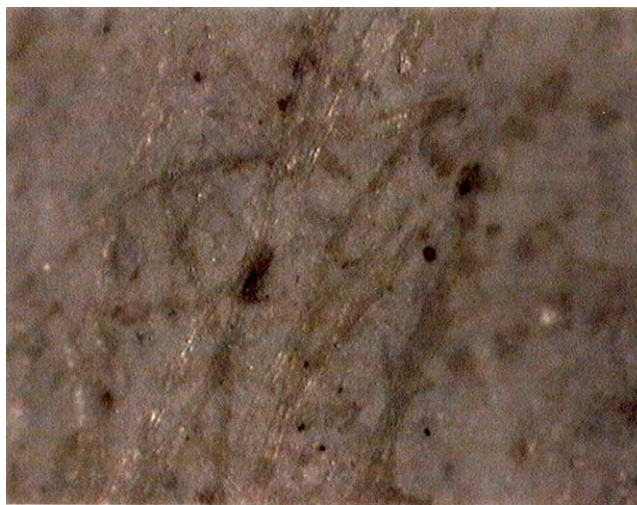
Fig. 1. Fibre alignment on the surface of a Hatschek made fibre cement.
