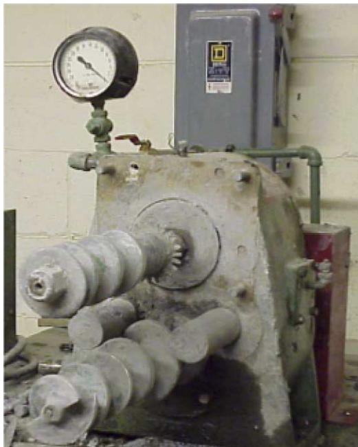
Fig. 2. The used auger extruder (with barrel removed).
