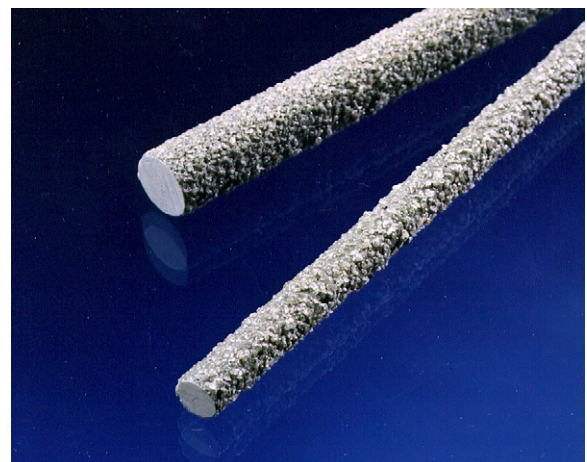
Fig. 1. Sand-coated glass FRP bars used in the current study.
