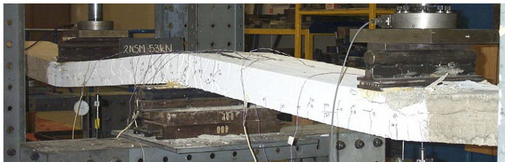
Fig. 7. Continuous beam with tension face NSM CFRP plates.
