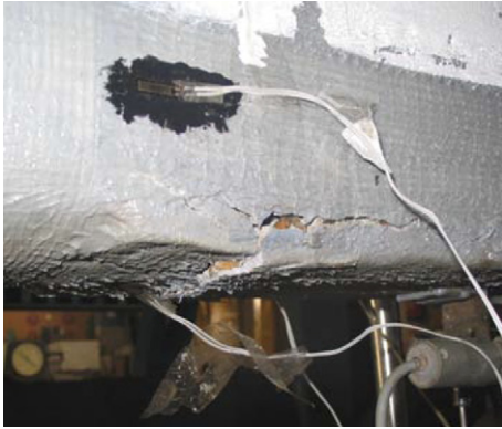
Fig. 11. Rupture of CFRP laminates without any damage in GFRP for specimen F06.
