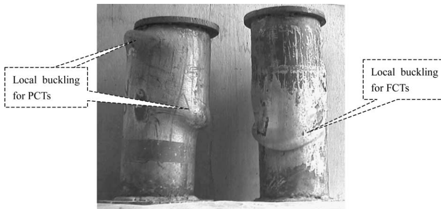
Fig. 4. Typical failure modes of CFT columns after 1 year curing.
