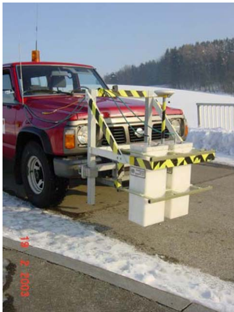
Fig. 7. EMPA's mobile acquisition system for pavements and bridge decks.
