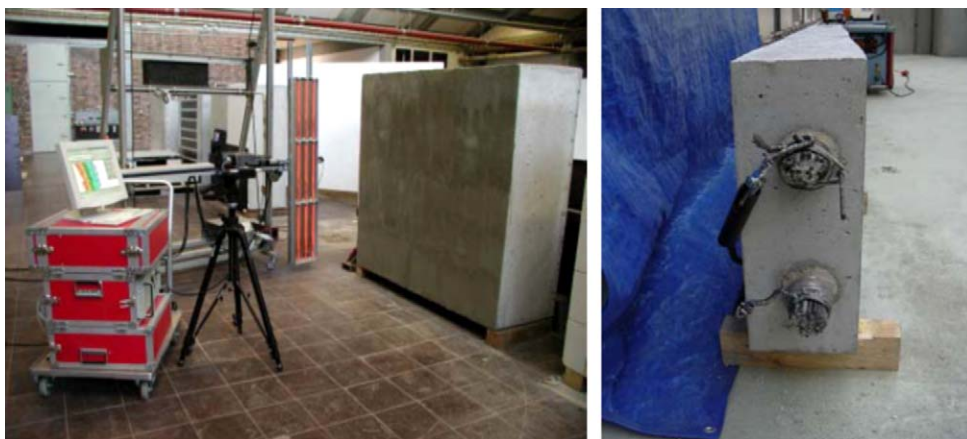
Fig. 1. Left: experimental set-up with infrared camera, computer and infrared radiator for direct heating of the surface. Right: electrical connections at the wires inside the tendon ducts for indirect heating by electric resistance.
