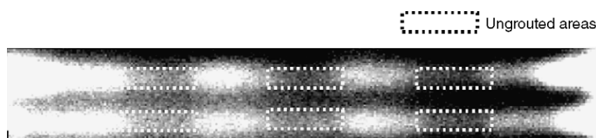
Fig. 11. Temperature distribution, 40 min after switching on of the heating source (white: temperature > 16.0 °C, black: temperature < 14.5 °C). The six ungrouted areas are colder than the grouted areas of the two horizontal tendons.
