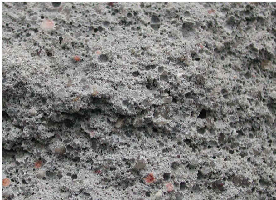
Fig. 7. Appearance (enlargement of approximately 30×) of mortar made with CEM I + 0.2% of protein additive.
