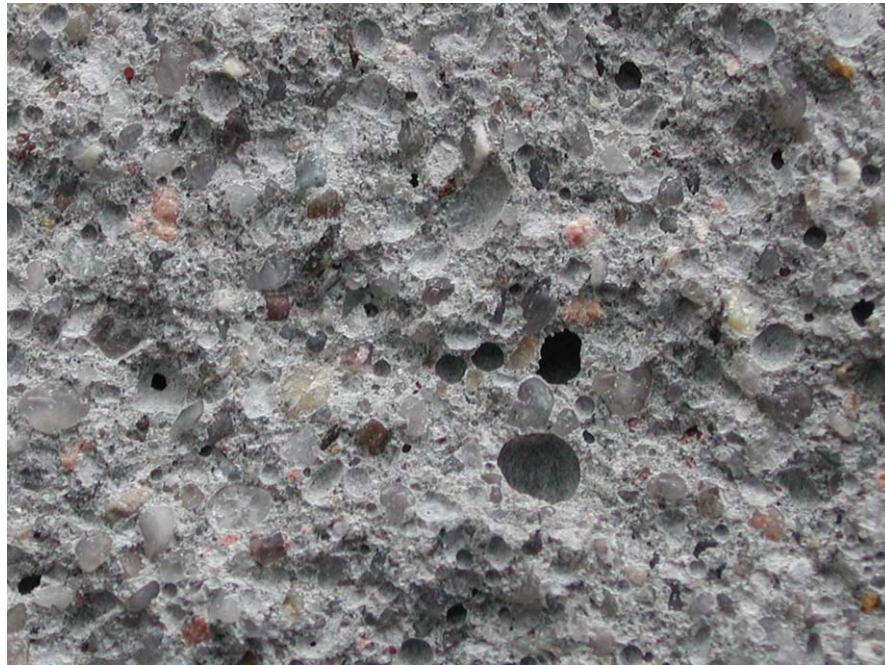
Fig. 6. Appearance (enlargement of approximately 30×) of mortar made with CEM I.
