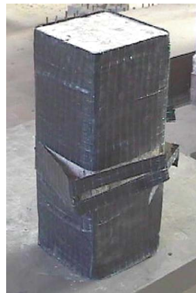
Fig. 3. Failure mode of CFRP continuously wrapped specimens.
