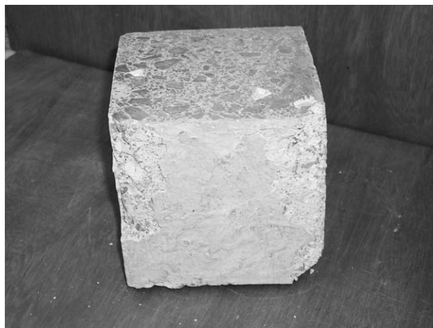
Fig. 2a. Mixture M-3. Noteworthy damage after freezing and thawing cycles.
