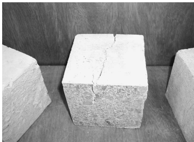
Fig. 2b. Mixture M-5. Cracked sample after freezing and thawing cycles.
