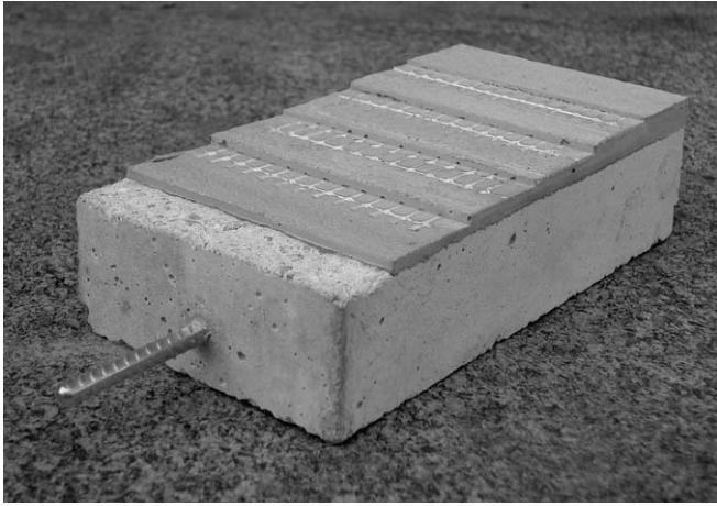
Fig. 1. Example of textile reinforced concrete.
