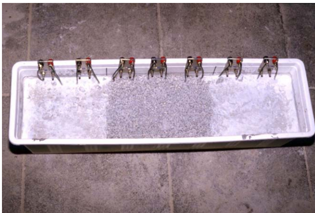
Fig. 3. Specimen for the simulation of a patch repair.
