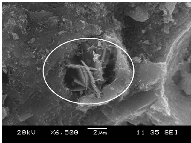
Fig. 13. Micrograph of HH/300-Y mortar (monosulfate formation at early age).
