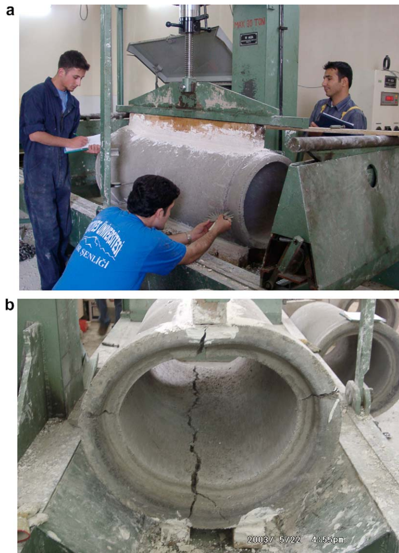
Fig. 2. (a) Three-edge-bearing test applied on one of the pipes. (b) The crack formation of a steel fiber concrete pipe under three-edge loading.
