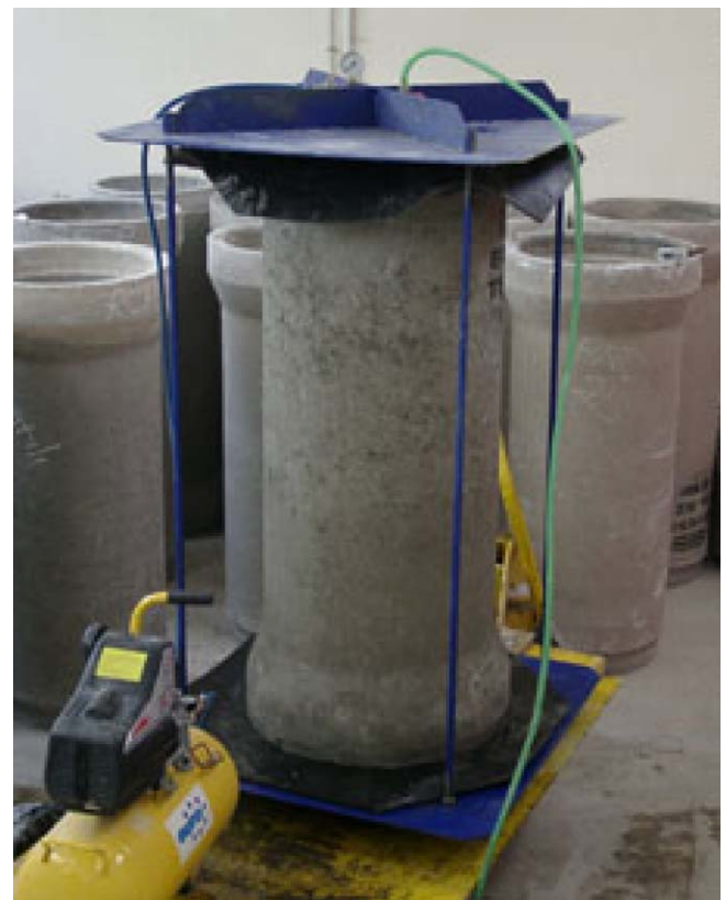
Fig. 3. Water-tightness experiment applied to one of the pipes.
