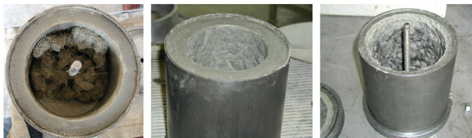
Fig. 12. Fiber segregation effects after centrifugation (laboratory setup) left: L8 (PVA-2), middle: L5 (PVA-1), right: L1 (carbon).
