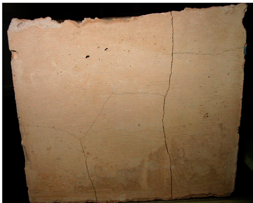
Fig. 6. Cracking due to drying on a MS100 beam kept in controlled atmosphere (after 1 month).
