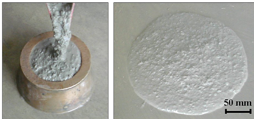
Fig. 3. The mini-slump flow testing of SCRM.
