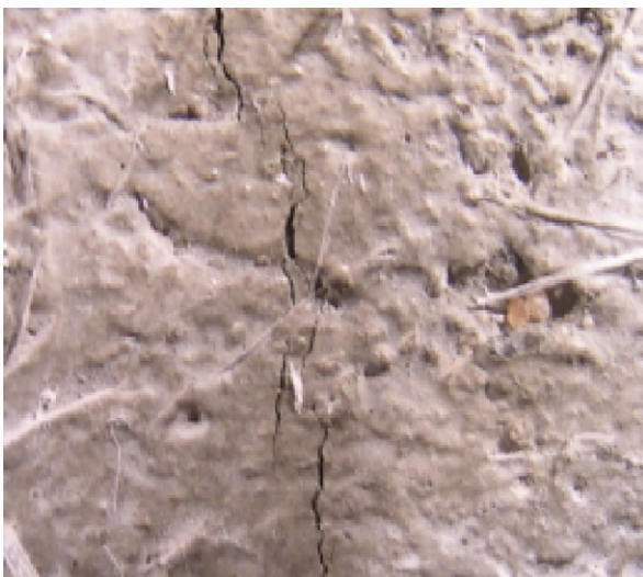
Fig. 5. Plastic shrinkage crack in the steel–polypropylene hybrid concrete (HSPP3) slab (area 35 \times 35 mm).
