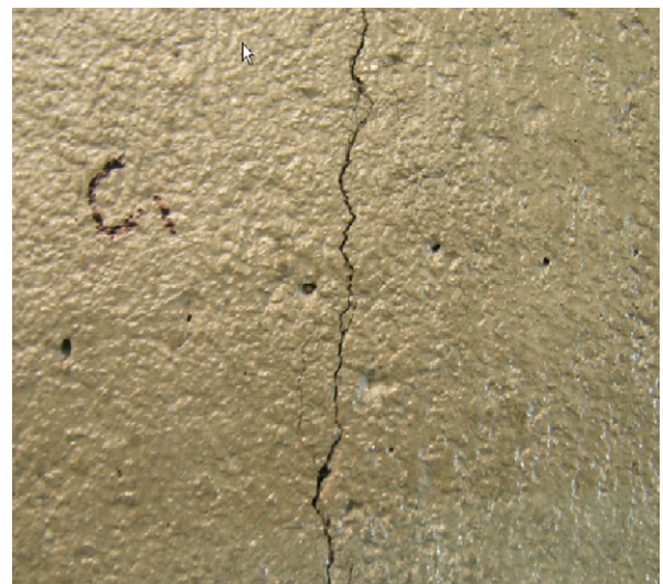
Fig. 3. Plastic shrinkage crack in the plain concrete (C1) slab (area 250 \times 250 mm).
