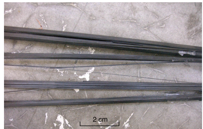
Fig. 6. Failure mode of the CFRP rod in tension.
