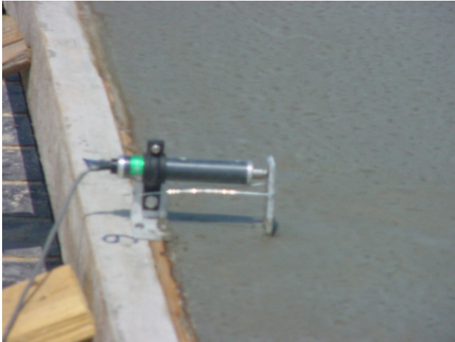
Fig. 2. Close up view of the LVDT used for plastic shrinkage strain measurements.
