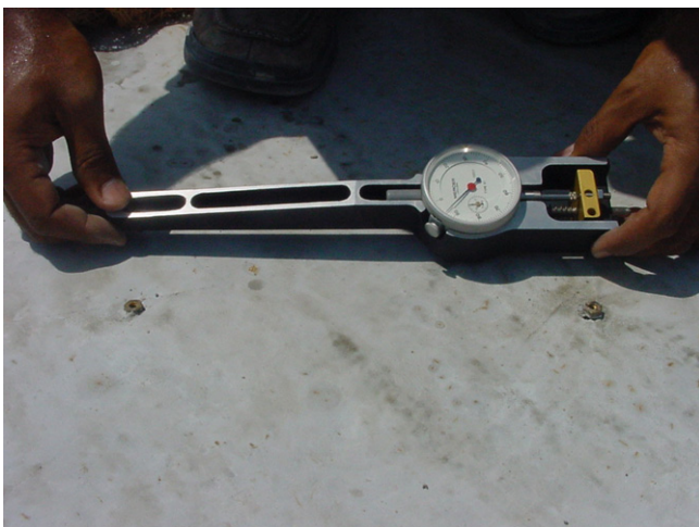
Fig. 3. Measurement of drying shrinkage strain using an extensometer.
