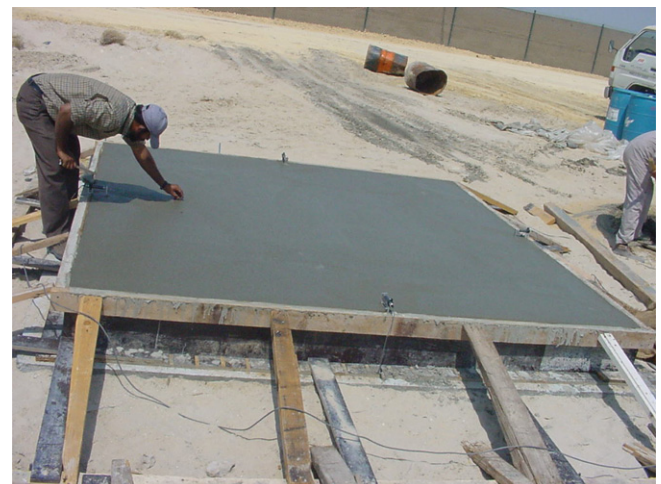
Fig. 1. Concrete specimen with LVDTs for measuring the plastic shrinkage strain.
