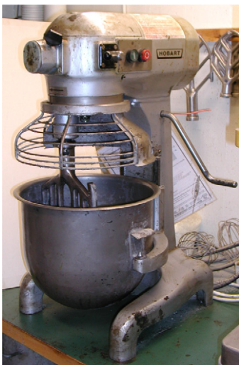
Fig. 4. Hobart mixer equipped with a paddle stirrer.
