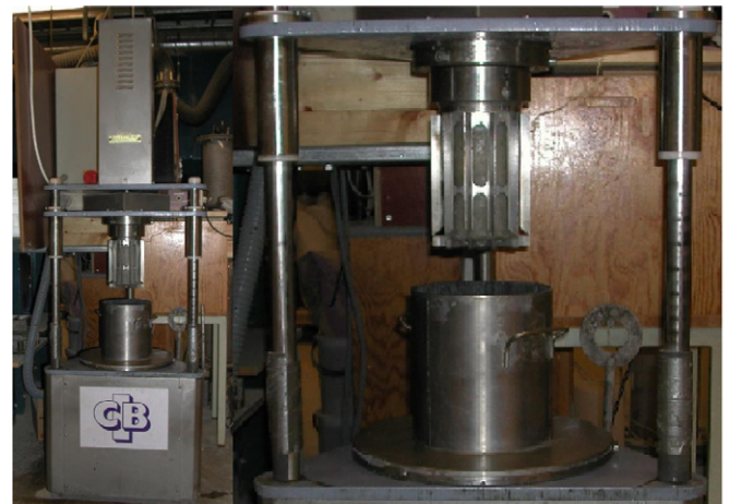
Fig. 5. Viscometer, Contec 4, with concentric cylinders used for characterization of mortars.
