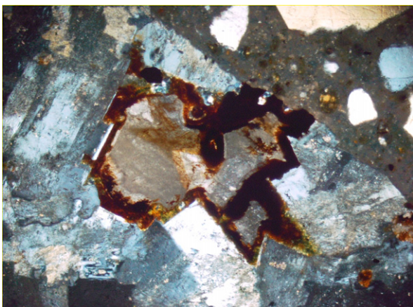
Fig. 12. Peripheral oxidation of siderite on outer surface of aggregate, WOF = 1.75 mm, XPL.
