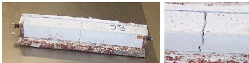
Fig. 6. Drying shrinkage cracks within the moulds.
