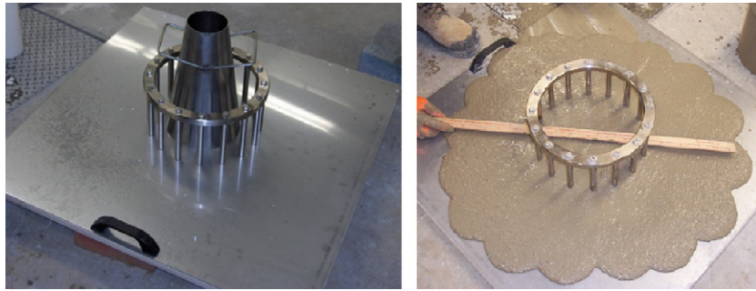
Fig. 1. Cone slump flow of CLSM with J-ring.
