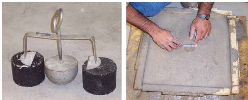
Fig. 3. Ball drop apparatus and test measurement for CLSM.
