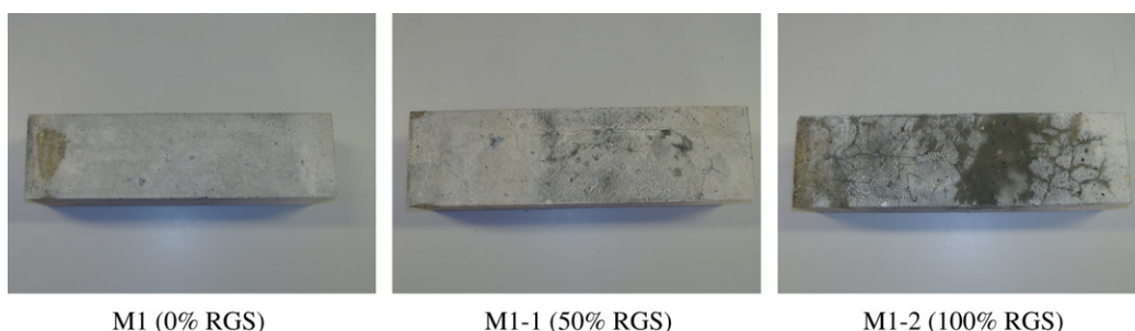
Fig. 5. ASR cracks in concrete mixes – group 1. No ASR suppressors were used.
