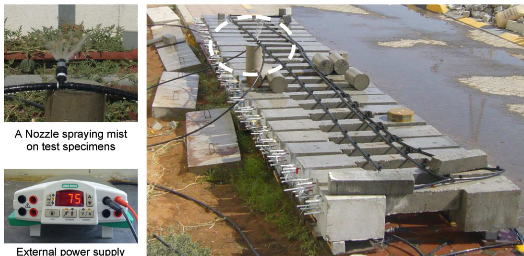
Fig. 2. Accelerated corrosion exposure.
