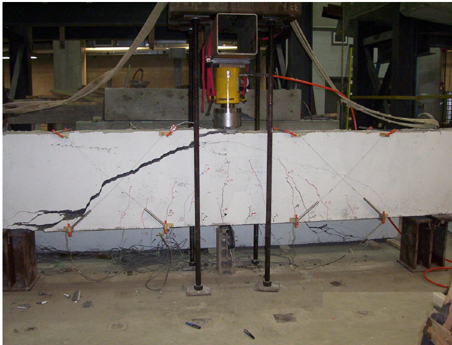
Fig. 3. Test setup, instrumentation and testing and failure mode of a beam specimen.
