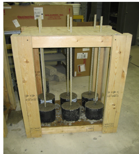
Fig. 3. Setup for fabrication of pullout specimens.
