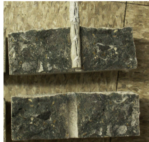
Fig. 7. Concrete bond failure of pullout test [2].
