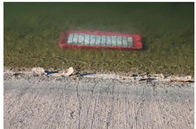
Fig. 5. Placement of samples in the Arizona canal.
