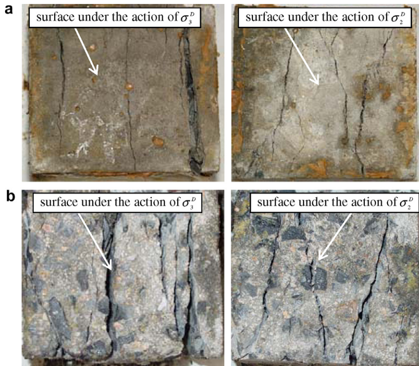
Fig. 2. The failure mode and surface cracking of specimen: (a) 0 cycles of freeze–thaw; (b) 300 cycles of freeze–thaw.
