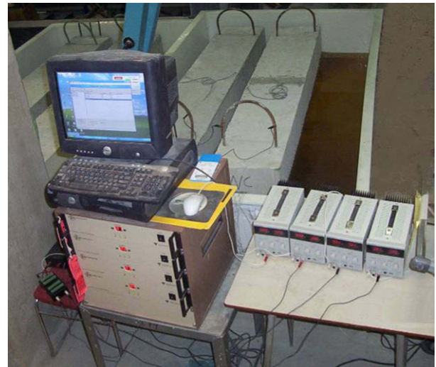
Fig. 2. Corrosion current monitoring by data-acquisition system.
