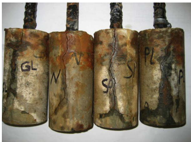
Fig. 11. Corrosion performance in the small concrete cylinders.
