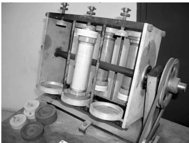
Fig. 2. Device intended to prevent the fresh cement paste segregation by slow rotation.
