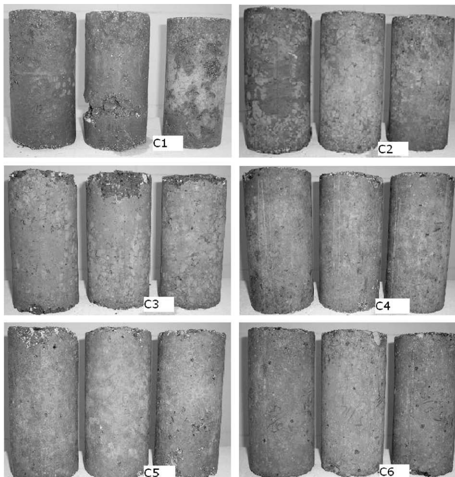
Fig. 5. MEPS concrete samples after 300 cycles of freezing–thawing.
