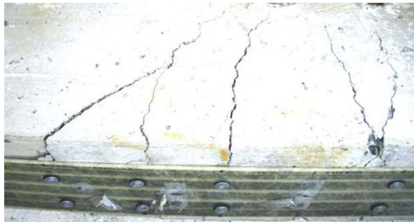
Fig. 7. Photograph of flexure cracks near midspan in relation to the nail locations.
