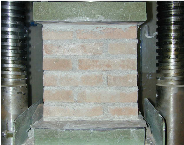
Fig. 10. Masonry assemblage for compression test.
