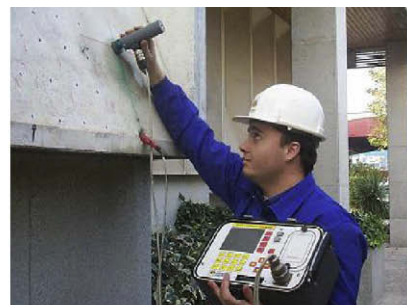
Fig. 1. (a) Corrosion risk map of a reinforcement slab calculated from the combination of E_{\text{corr}} and \rho measurements; and (b) on-site measurement with a portable corrosion rate meter (Gecor 08).
