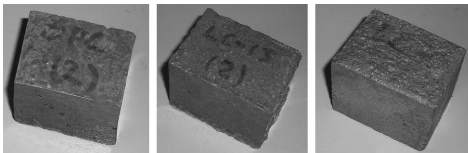
Fig. 4. Specimens with calcreous sand cured for 60 months in a 1.8% \text{MgSO}_4 solution at 25 °C.
