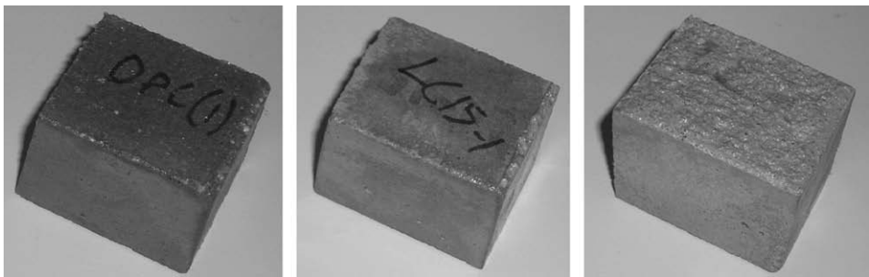
Fig. 3. Specimens with siliceous sand cured for 60 months in a 1.8% \text{MgSO}_4 solution at 25 °C.
