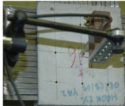
(b) LVDT attached to middle point of the back of the panel to measure out-of-plane expansion
