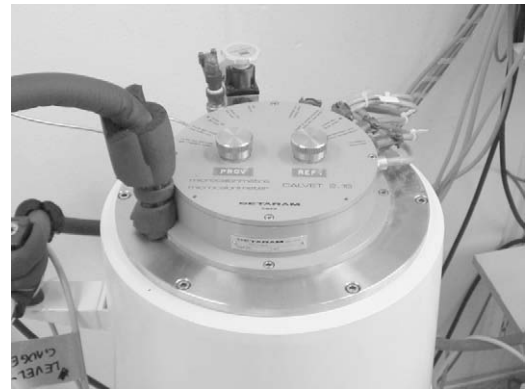
Fig. 1. Top of the SETARAM scanning calorimeter showing the liquid nitrogen supply tube and the reference and sample container.
