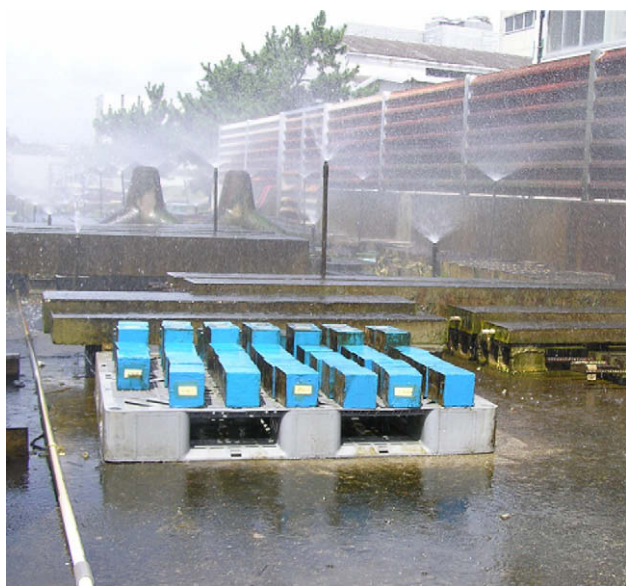
Fig. 4. Exposure of specimens subject to cyclic sea-water shower.
