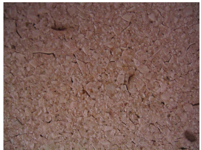
Fig. 5. Digital camera picture of specimen surface exposed to 1200 °C.
