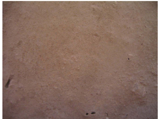
Fig. 4. Digital camera picture of specimen surface exposed to 1000 °C.
