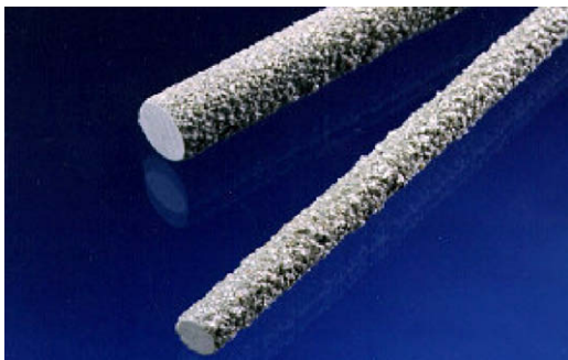
Fig. 1. Surface configuration of a GFRP bar.
