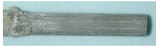
Fig. 6. Details of the embedded length after failure.
