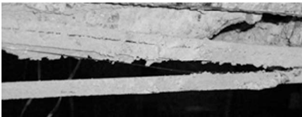
Fig. 18. Appearance of the NSM strips at the end of the test.
