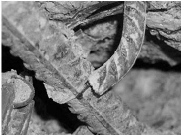
Fig. 17. Sliding of the central stirrup in the L_1 span (VL3 beam).
