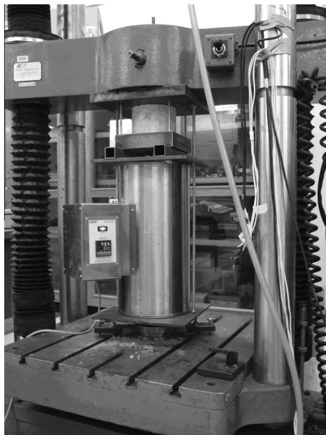
Fig. 1. Test equipment-loading frame with furnace.
