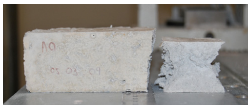
Fig. 7. Mortar compactness data for Series I and picture of specimen I-100 after compressive strength testing.
