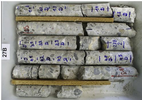
Fig. 3. Cores taken at coring site 27B. On the left side, the concrete is exposed to air. On the right is the contact to the rock face.
