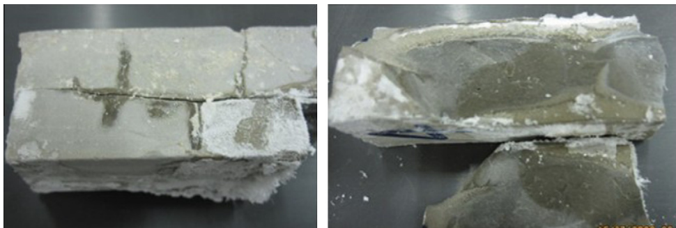
Fig. 2. Visual observation of cement paste specimen exposed to sodium sulfate solution.
