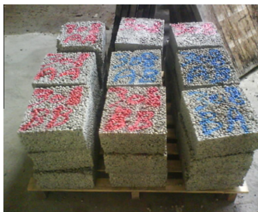
Fig. 10. Appearance of manufactured concrete masonry units.
