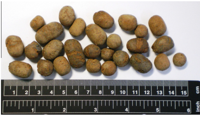
Fig. 5. Appearance of sintered sedimentary LWA.
