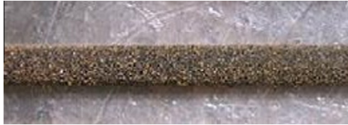
Fig. 1. Sand coated CFRP rods used in the study.
