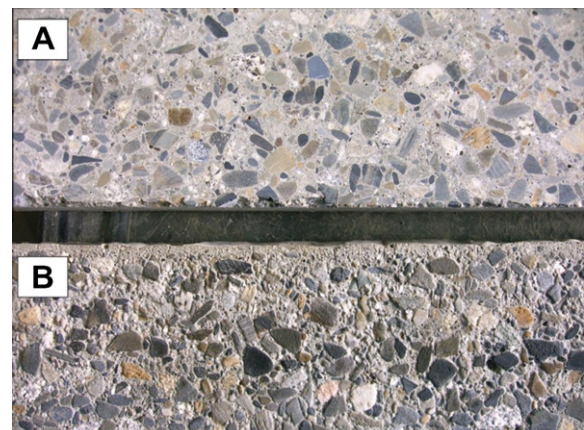
Fig. 7. Comparison between smooth (A) and sandblasted (B) concrete surfaces.
